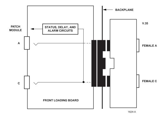
Figure 3-2. V.35 Interface Module and Conversion Board
